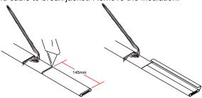
6. Shave off out matrix material from each bus wires with a utility knife.
