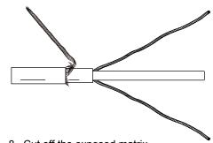
8. Cut off the exposed matrix. DO NOT CUT THE BUS WIRES.
