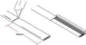
3. Move braid back toward the overjacket, creating a bulge. At the bulge, separate the braid to make an opening.
