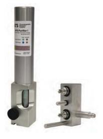
A high-capacity gas purifying system that removes oxygen, moisture and hydrocarbons, (greater than C4) from inert gases and hydrogen. It contains a high-sensitivity oxygen and moisture indicator. When the cartridge is depleted the oxygen indicator changes from GREEN to GREY and the moisture indicator changes from BLUE to BROWN. The AFS Purifier I can be expected to supply multiple GC installations for an extended period of time depending on the laboratory environment.
