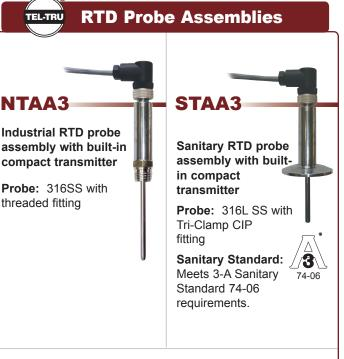
4 to 20 mA 2-wire loop powered output, with single element thin film Pt100 3-wire RTD, Accuracy Class A +/- .06% at 0°C (coefficient 0.00385)
