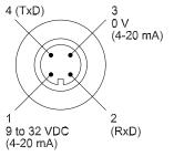
AXX Wiring Models NT100 and ST100 1 = Red 3 = Black Electrical connection of the compact thermometer (view from above) – M12 plug, 4-pin Pin 1: Power supply 9 to 32Vdc; Current output 4 to 20mA
