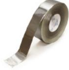
AAT2180 | <b>High Temperature Aluminum Tape</b><br>Designed for applications above 392°F (200°C)<br>Size: 2 in x 180 ft (51 mm x 55 m)<br>Silicone Adhesive w/Liner<br>Temp Limit: 550°F (288°C)        |
