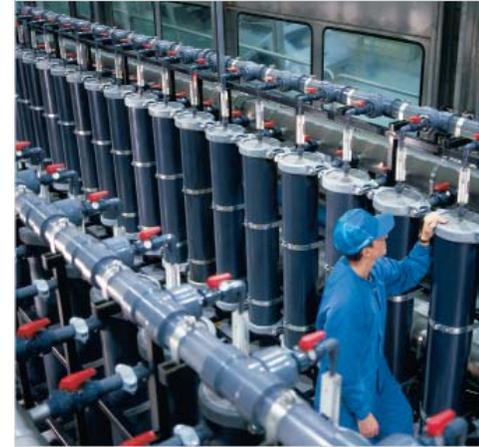
Designed for extended life in a wide range of industrial and electrocoat applications, EP Ultrafiltration Spiral Elements provide greater resistance to fouling by colloidal particles and oily contamination. The Polyvinylidene Fluoride (PVDF) membrane provides excellent chemical and temperature resistance under a variety of process conditions.
