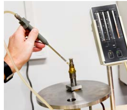
Helium mass spectrometer for leakage rate measures
