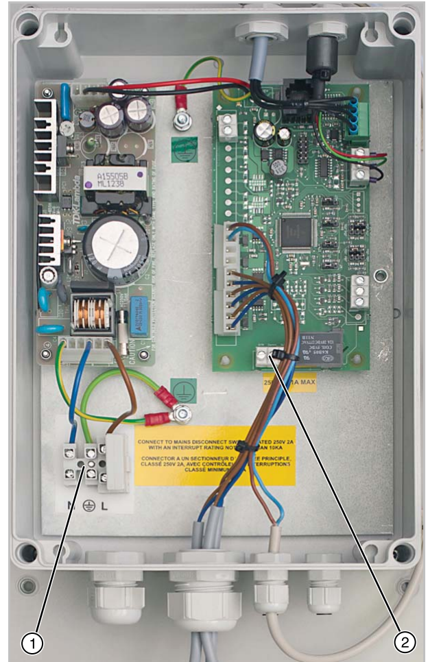
1 Electrical supply terminal block: 2 Remote alarm terminal block
