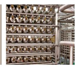
Reverse Osmosis (RO) sanitary spiral elements are designed to provide extended life in a wide range of food processing and dairy applications. The high-rejection membranes are well-suited for processes requiring dewatering or product concentration.
