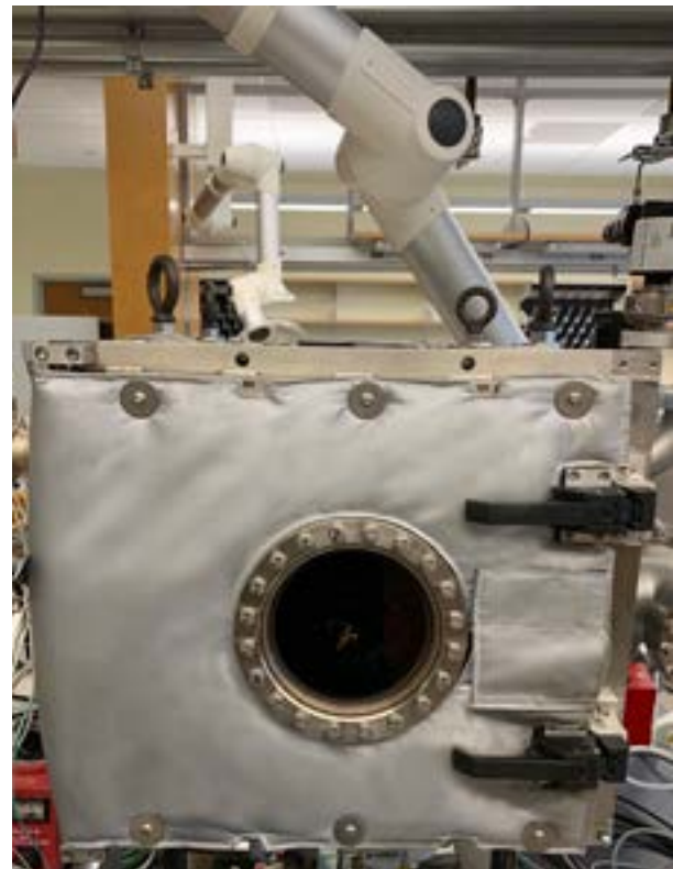
Silicone Cloth Vacuum Chamber
