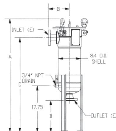
(3) 9/16" x 7/8" SLOTTED MOUNTING HOLES SPACED ON A 7.00" B.C.D.
