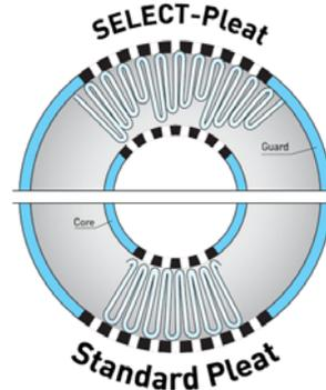
With Select Pleating, there is more open area on the inside of the cartridge for additional contaminant-holding capacity.
