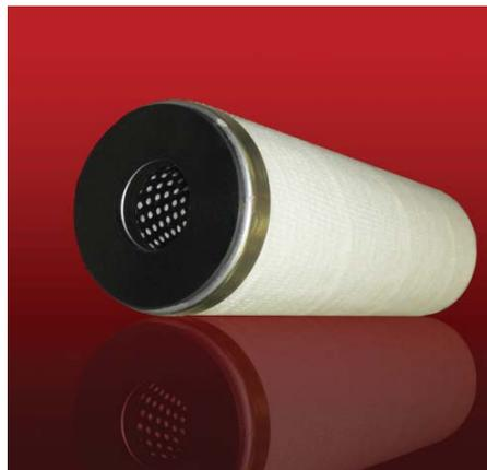
The all synthetic Fulflo® LC Hydrocarbon liquid-liquid coalescers utilize a proprietary, high performance coalescing media in a pleated configuration to improve performance. The liquid-liquid coalescers are designed to remove water from hydrocarbons or hydrocarbons from water.
