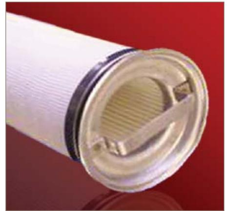
Parker domnick hunter's high performance Naphtha Coalescer is designed to remove water from light naphtha or heavy naphtha. The proprietary Nylon 66 coalescing media is designed specifically for naphthas, aromatics and hydrocarbon solvents. Because naphthas contain higher ratios of aromatics and may be treated with caustics, common materials of construction used in coalescing elements often are not compatible with naphtha.
