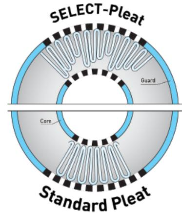
With Select Pleating, there is more open area on the inside of the cartridge for additional contaminant-holding capacity.
