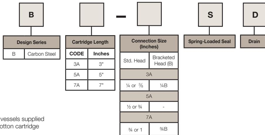
Note: B3A, B5A and B7A vessels supplied with 10µm Fulflo wound cotton cartridge
