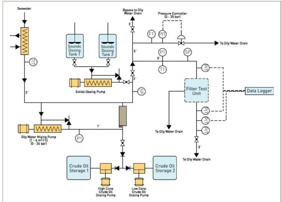
Figure 2 - Test Stand Schematic
