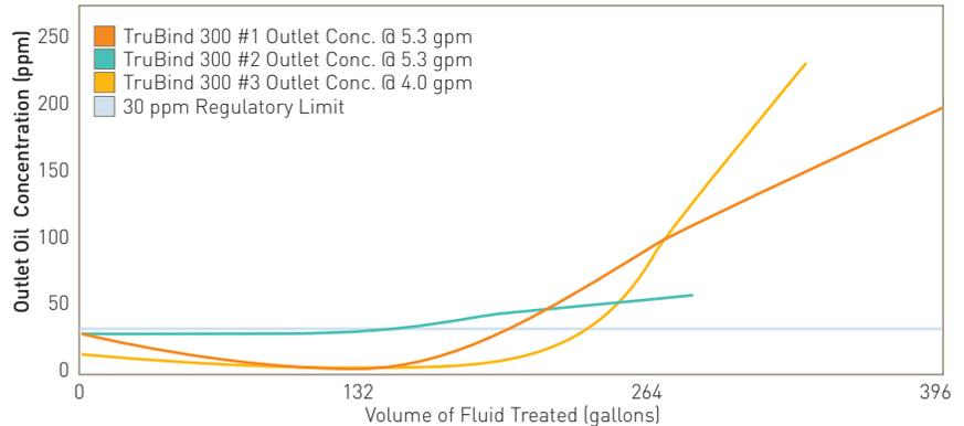
Graph 3 - TruBind 300 Effect of flow rate on mass of oil removed
