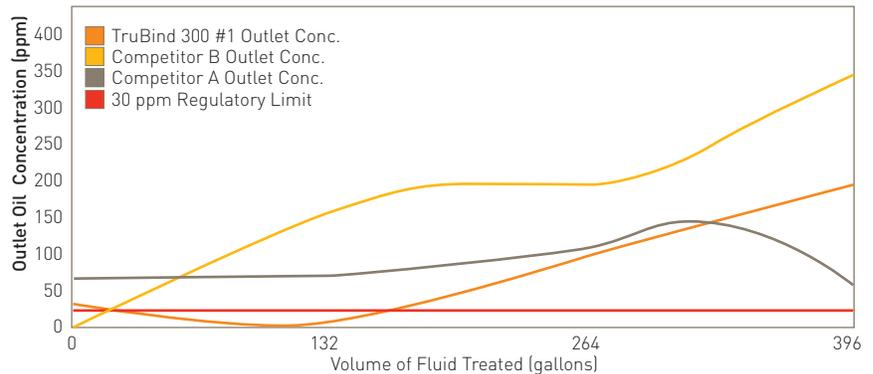
Graph 5 - Competitive comparison mass of oil removed at 5.3 gpm
