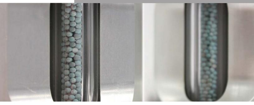
A high-capacity gas purifying system that removes moisture and hydrocarbons, (greater than C4) from air, inert gases and hydrogen. It contains a high-sensitivity moisture indicator. When the cartridge is depleted the moisture indicator changes from BLUE to BROWN. The AFS Purifier II can be expected to supply multiple GC installations for an extended period of time depending on the laboratory environment.
